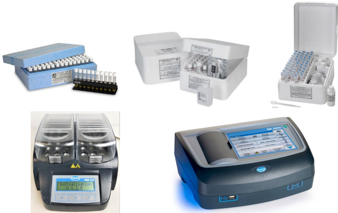
Figure 9. (up) Water quality analysis kits for the COD and nutrient measurements, (down-left) HACH DRB 200 sample digester, (down-right) HACH DR3900 UV-Visible spectrometer
