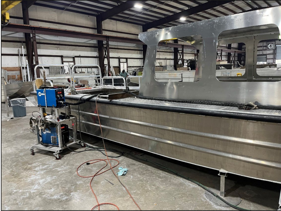
Appendix Figure 3. Construction progress on new Turtle Cove 30' Aluminum Cabin Workboat that will be used to assist in LMM buoy deployment, and which will be made available to all research teams as needed. Funds for the purchase of this Workboat came from an external source (non-LMM funds).
