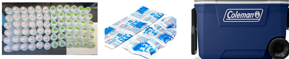
Figure 5. (left) Sample bottles used for the collection of water and sediment samples, (middle) Dry ice, (right) Ice chest for safe transportation of the collected samples.
