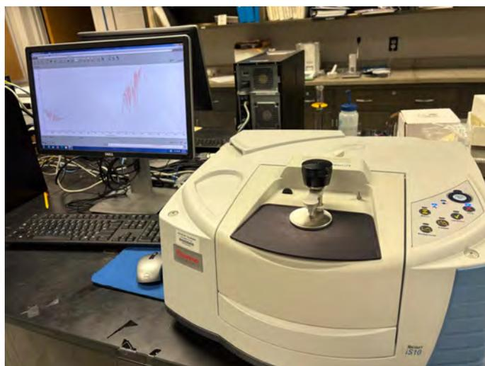
**Figure 8.** Fourier Transform Infrared Spectroscopy (FT-IR) for chemical characterization of MPs.
