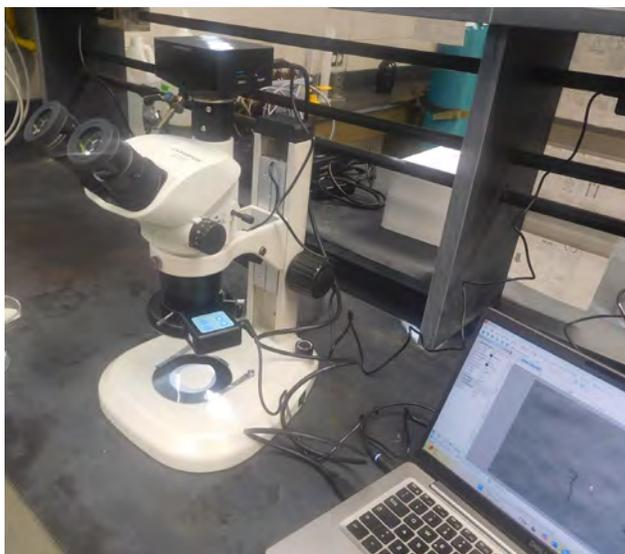
**Figure 7.** Stereo microscope with attached camera for MPs quantification.
